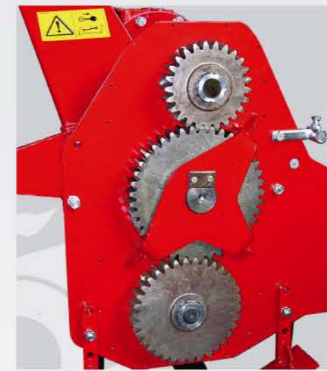
Bočni zupčasti prenosnik, nosač u obliku "Y" stabilizuje srednji zupčanik Side toothed drive, the support in a shape of a "Y" stabilizing the middle cog wheel
