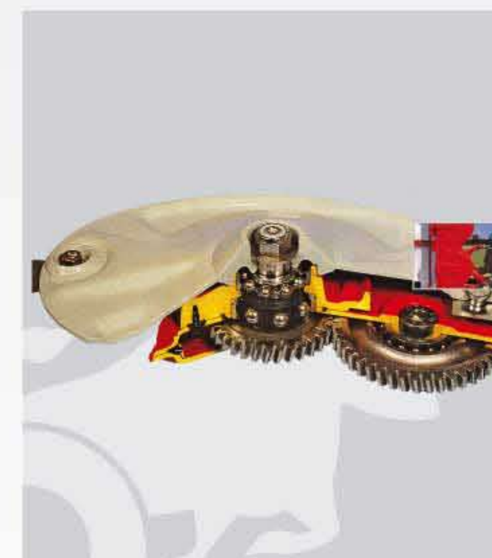
Detalj preseka reznog aparata. Cross section detail of the cutter bar.
