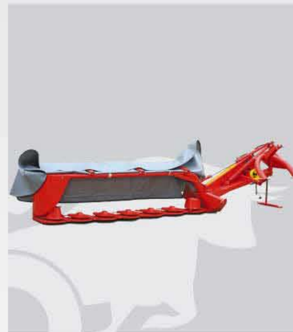
Izgled kosačice pre prikačivanja na traktor Overview of the mower before connecting on tractor
